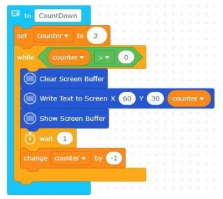
When we call the function, let's determine it by dragging it into the function block for it to print X=60 Y=30 coordinates 3-2-1 on the OLED screen.
