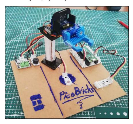
12. You can operate the Robot arm if you feed Picobricks with USB or 3 pen batteries from the power jack on the Picoboard.
