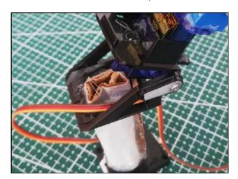
10. Put the motor drive jumpers on the Servo pins. Connect the cable of the holding servo to the GPIO21 and the cable of the tilting servo to the GPIO22.
