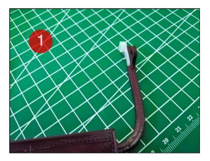
1: Fix the plastic apparatus of the servo motor to the piggy bank arm with 2 screws.
