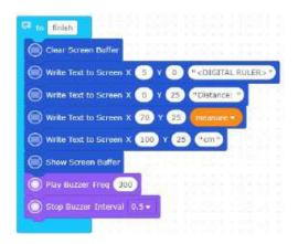
Let's call the functions we made by using the loop and condition structures. Make the measurement every time the button is pressed and print the value of the measurement on the OLED screen.
