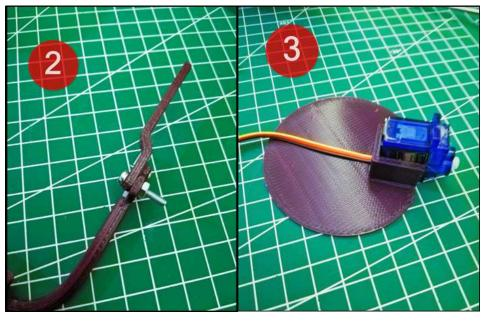
2: Fix the second part of the piggy bank arm with the M3 screw and nut to the first part where the hopper is.
