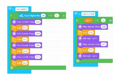
■ Call these functions by using the condition and loop structures. Connect PIR sensor to GPIO 14 and GAS sensor to GPIO 16 digital pins. Create the code blocks call the "GASControl" and "PIRControl" functions, if the values from Gas and PIR sensors are "1".
