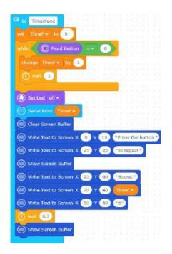
Let's drag the code blocks that provide to print "TimeF" variable on the OLED screen when the button is pressed, otherwise to increase the value of "TimeF" variable one by one, into the function block. When you call the function, a timer will run and it will stop when the button is pressed and print the score on the screen.
