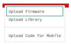
After opening PicoBricks IDE, click the PicoBricks menu and then, click "Upload Firmware" tab from PicoBricks Menu. In the window that opens, you should put PicoBricks into Bootsel mode.
