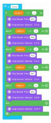
■ Let's play the notes according to the distance value with buzzer, by using "Forever" loop block.
