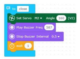
Let's define the code blocks that, set the position of the servo motor to lean robot arm down into the "down" function.
