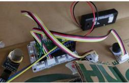
When you connect the battery case to Picoboard and open it, the codes will start to run. 3 seconds after pressing the button, the alarm system will be activated and the red LED will turn on. As soon as you put your hand in the door, the buzzer will start to sound.
