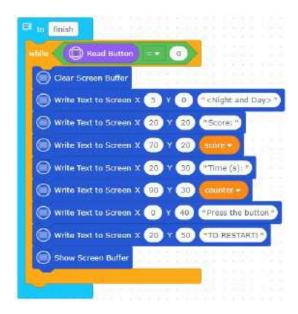
Let's create the code block structure by using the loop and condition structures that call the functions. Let's create a structure that randomly generates numbers between 1 and 2, prints "NIGHT" on the screen when the number is 1, and prints "DAY" on the screen when the number is 2, measures the value of LDR according to the value and determines the score of the player.
