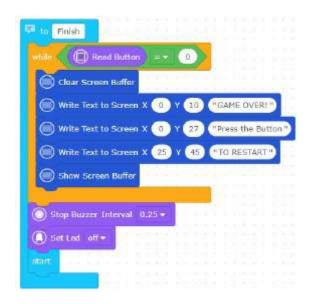
Let's call the functions created by using the necessary condition and loop structures. Create the code blocks that, run buzzer, turn on LED and call the "finish" function if the value from GPIO 01 pin is "0".
