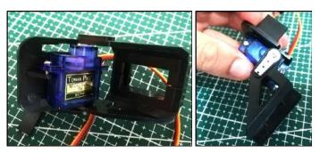
5. For the holder, cut one of the servo motor heads in the middle of the gear part that you printed on the 3D printer and place it into the gear. Then screw it to the servo motor.
