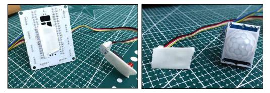
Place pieces of Picobricks inside the model house. Position the PIR sensor to see the
