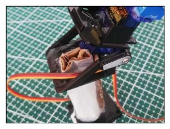
10. Put the motor drive jumpers on the Servo pins. Connect the cable of the holding servo to the GPIO21 and the cable of the tilting servo to the GPIO22.
