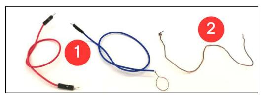
Bend the conductor wire on the protoboard as you wish and pass it through the holes, before passing one end, you must pass the male end, which is connected to the GND pin on the PicoBoard, the other end of the cable you have made into a ring.
