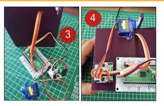
3: Pass the cables of the ultrasonic distance sensor through the hole in the box and connect them to the pins shown in the PicoBricks circuit diagram, make the servo motor and motor driver connections.
