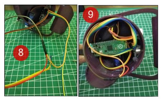
8: Plug the cables of the servo motor and ultrasonic distance sensor and connect the power cables.
