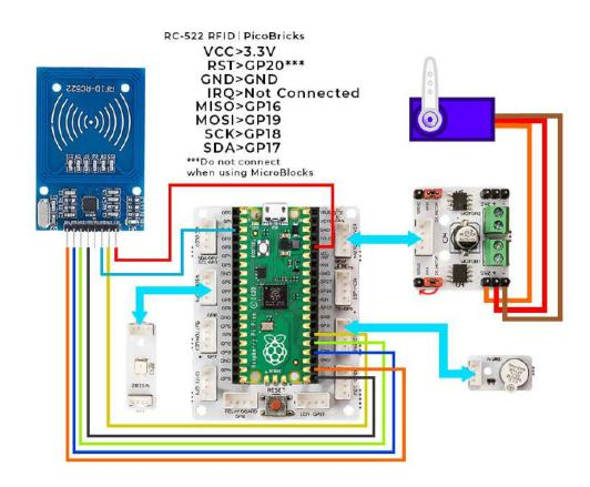
Be sure to make the cable connections of the RC522 RFID card reader module according to the table below.
