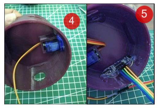
4: Place the servo motor and its housing on the body of the piggy bank. You can use hot glue here.
