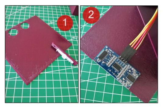
1: Fix it by screwing it to the trash bin cover of the servo motor apparatus.
