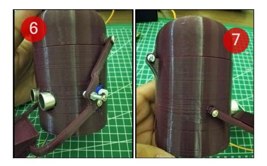
6: Attach the piggy bank arm to the servo motor and fix it to the top cover with M3 screws.
