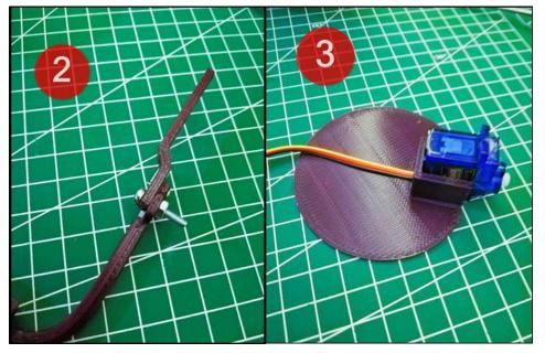
2: Fix the second part of the piggy bank arm with the M3 screw and nut to the first part where the hopper is.
