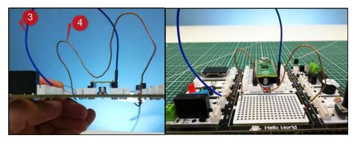
5: One end of the jumper cable, which has both male ends, into the hole right next to the end of the conductive wire you placed on the protoboard
