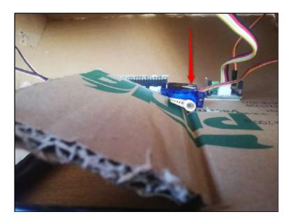
Finally, place the Pico board and the 2-key battery box inside the model house and complete the cable connections. After making the final checks of your project, it is ready to work.
