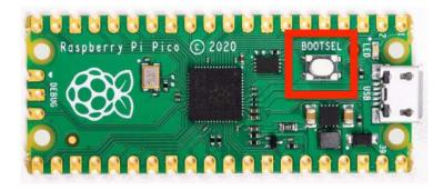
In this way, Pico will be connected in bootloader mode and recognized by your computer as external memory. Connect Pico to your computer by holding down the Bootsel button. After seeing Pico as the computer's flash memory, activate your card by going to **Tools>Board>Arduino Mbed OS RP2040 boards> Raspberry Pi Pico**.
