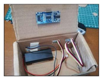
3. After completing the cable connections of all modules, you can insert the 2-battery box into the power jack of the Picoboard and turn on the switch. That's it for the digital ruler project!
