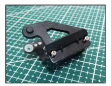
4. Internally attach the servo motor to part C. Then place the servo motor on part B and screw it.
