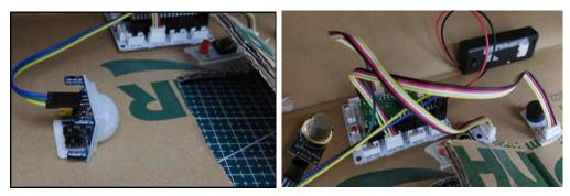
When you connect the battery case to Picoboard and open it, the codes will start to run. 3 seconds after pressing the button, the alarm system will be activated and the red LED will turn on. As soon as you put your hand in the door, the buzzer will start to sound.
