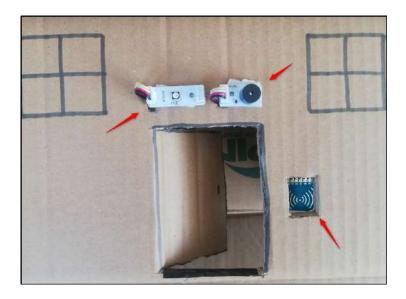
Attach the servo motor to the inside of the model with double-sided tape as a hinge in the upper left corner of the door. Attach the servo head to the door with hot glue or liquid glue.
