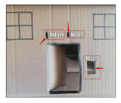
Stick double-sided foam tape on the back of the RGB LED and Buzzer and stick it on the box. Place the RC522 inside the model as in the image.
