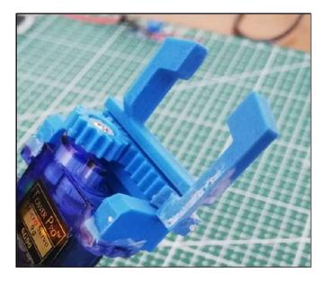
8. Stick the holding servo system to part B with silicone.
