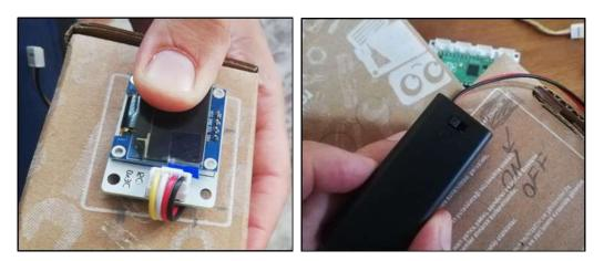
2. Hang all the cables inside the box and stick the back of the modules to the box with double-sided foam tape. Connect the trig pin of the ultrasonic sensor to the GPIO14 pin and the echo pin to the GPIO15 pin. You should connect the VCC pin to the VBUS pin on the Picoboard.
