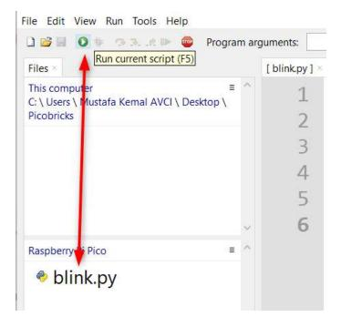
After seeing the "blink.py" file in Pico's file explorer, click the F5 key on the keyboard or the green Run button on the toolbar, and the code file will be run by Pico. If you see the internal LED on the Pico blinking at 1 second intervals, you have successfully written and run your first code. Congratulations :)
