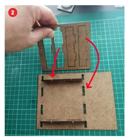
3- Remove the inner walls of the greenhouse from the SR-4 part and attach it to the ground of the greenhouse.
