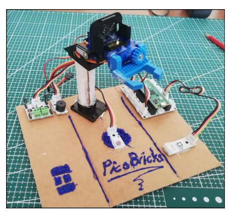
12. You can operate the Robot arm if you feed PicoBricks with USB or 3 pen batteries from the power jack on the Picoboard.
