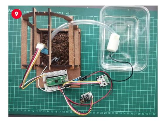
10- Plug the Soil Moisture sensor to the pin number GPIO27 on the Picoboard and connect the 2 pen battery to the power input of the Picoboard. Place the submersible pump and the end of the hose in a deep container of water. Be careful not to get the motor drive wet.
